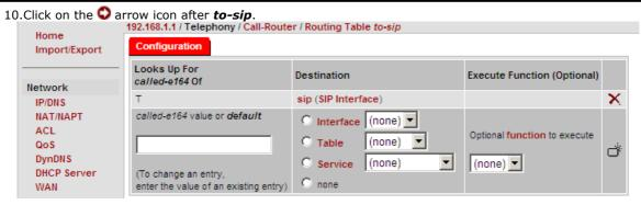
Ensure that the table contains T with the destination sip (SIP Interface).
