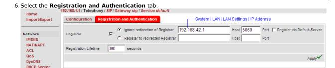
• Enable the Registrar checkbox. Select **Ignore redirection of Registrar** and enter the IP address and SIP port of the IP Office LAN on which the SIP registrar is enabled. Click **Apply** ✓.
