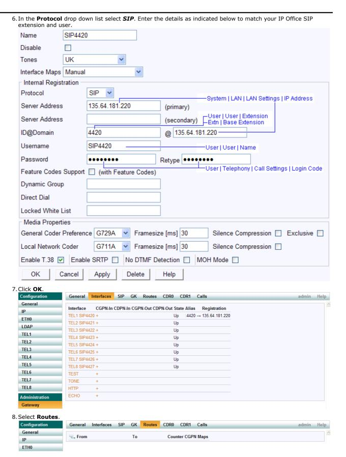
9. Two new routes are needed, one for dialing from the phone attached to the TEL port and one for incoming calls to the SIP account registered with the TEL port.
