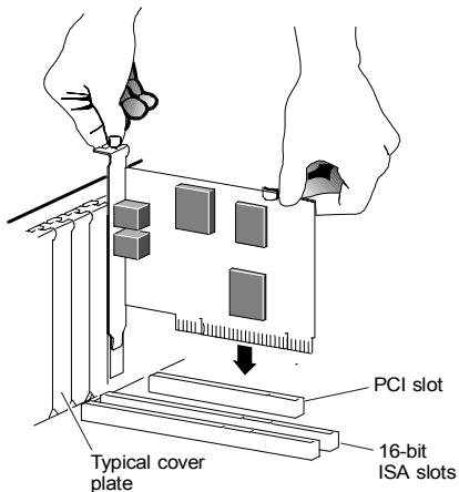
Be sure that the back end of the card (smaller gold finger area) is properly seated into the connector. If you have a tower or mini-tower computer case with a vertical main board, lay the computer down on its side so you can push straight down on the modem card to seat it firmly in its slot. Be sure that the bracket is lined up properly, then screw the bracket into the computer using the screw you removed earlier.
